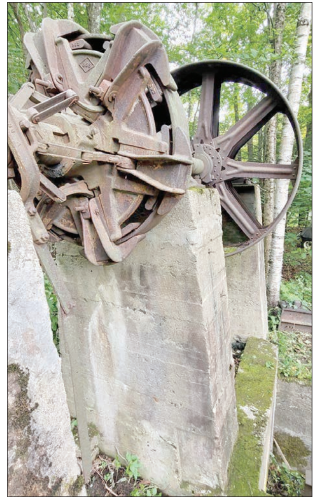
These belt driven wheels operated the saw.
