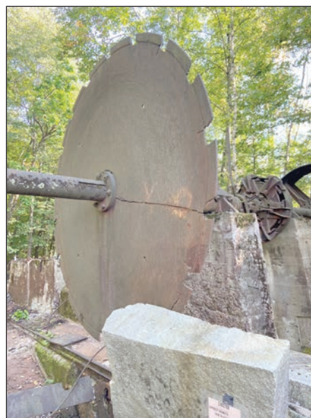
The 12 ft shot saw is still on site at the old Chester Hudson Granite Polishing Company.
