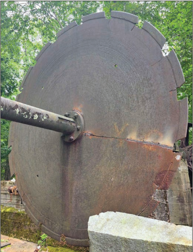
After the welding repairs, this is how the granite saw blade now looks.
