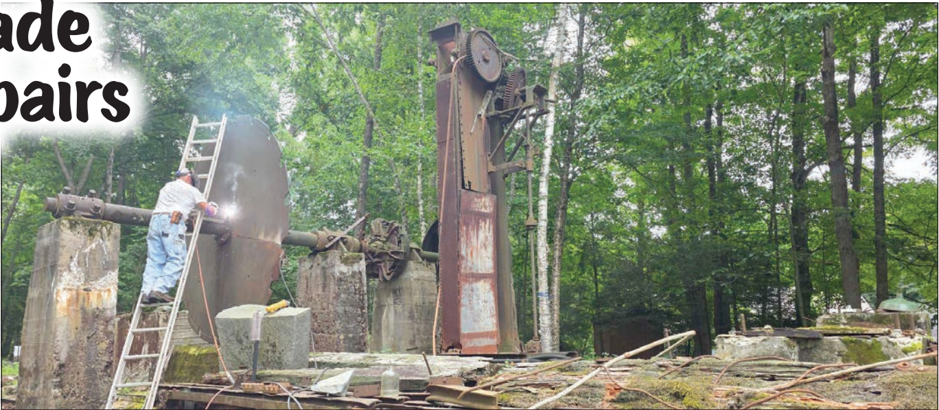
John Marcoulier stands on a ladder to weld the large granite saw blade.
