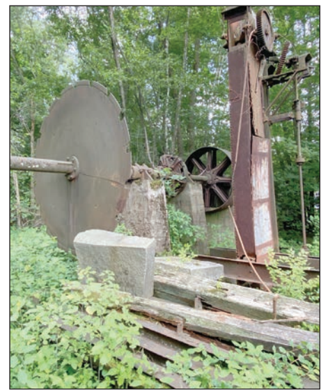
Granite cutting saw located in Chester, MA, that was used to cut Chester blue granite.
