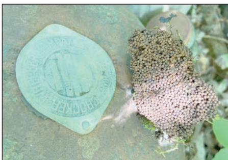
These shot pellets were used with the saw to cut granite. Photos by Deborah Daniels
