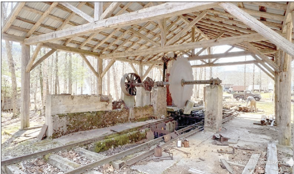
Here is another view of the giant granite saw with a pavillion protecting it from the weather.
