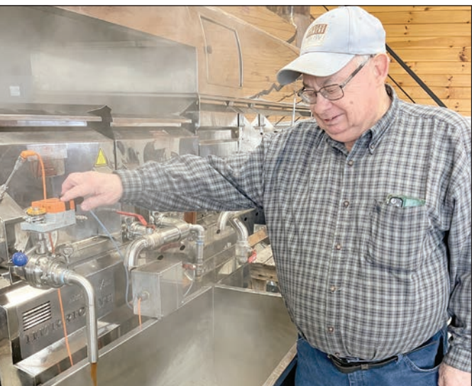
Leon Ripley turns the spigot to allow flow of boiled sap. The liquid is no longer clear, but amber colored.
